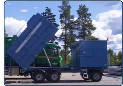
The SDT-20T suction units are equipped with built-in hydraulic tipping system and are towed/connected to i.e. a tractor
