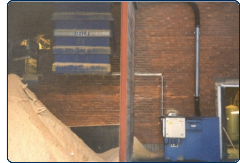
The PES 101 unit shall always be connected to a filter separator to complete a vacuum system
