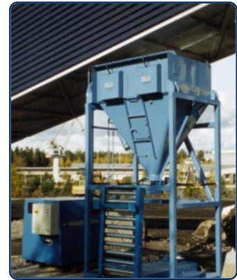
The BEASS filter containers shall be connected to a vacuum unit/power pack to complete a heavy duty vacuum system.
