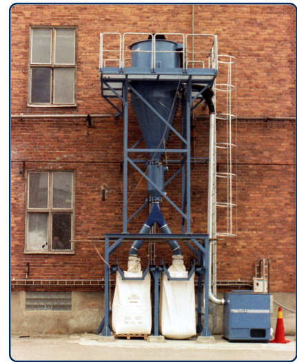
The BSAT filter containers shall be connected to a vacuum unit/power pack to complete a heavy duty vacuum system.
